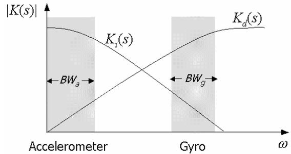
Fig. 3. Operating frequency region of the controller.
