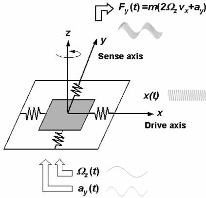
Fig. 1. Mechanical model of MEMS gyro-accelerometer.
