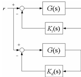
(b) Equivalent two closed loop in ID control.
