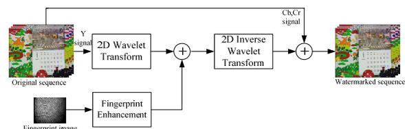
Fig. 1. The block diagram of the proposed watermark embedding procedure.
