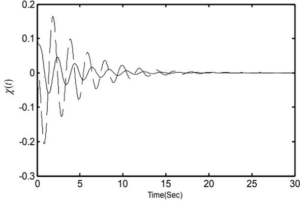
Fig. 3. The state responses  $\chi_1(t)$  (solid line) and  $\chi_2(t)$  (dashed line) for the closed-loop system where the initial states of the system (34) are  $\chi_1(0)=0.1$ ,  $\chi_2(0)=-0.2$ , and the initial states of the DRNN (32) are initialized arbitrarily.
