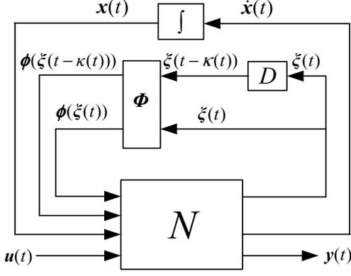
Fig. 1. Continuous-time standard neural network model (SNNM) with inputs and outputs.
