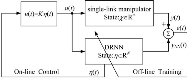
Fig. 2. The close-loop system of the single-link manipulator.
