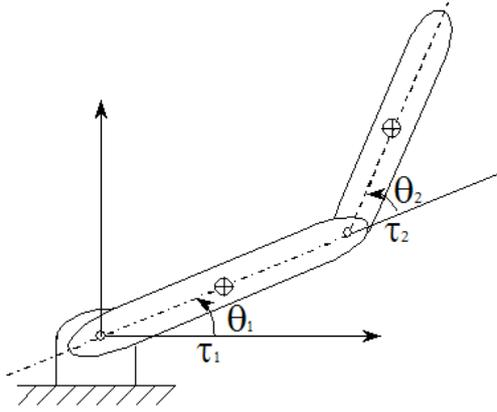
Fig. 2. An articulated 2-link robot manipulator.
