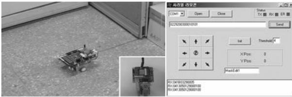
Fig. 8. Prototype robot for remote control test (left), Bluetooth host module (center bottom), and control panel (right).
