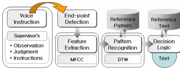
Fig. 2. Block diagram of voice recognition system.
