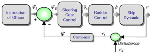
Fig. 6. Block diagram of steering control system.
