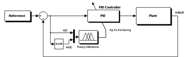
Fig. 1. Structure of self tuning PID controller.
