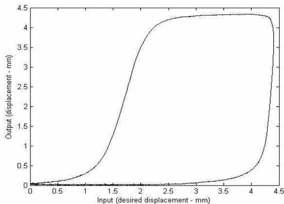
Fig. 19. Hysteresis curve obtained from experiment before applying control algorithm (open loop control).
