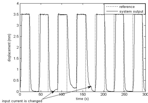
Fig. 18. Effect of the change of input current.
