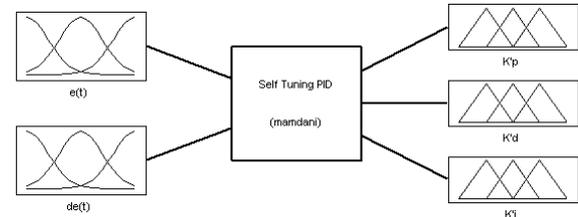
Fig. 2. Structure of the fuzzy inference block.
