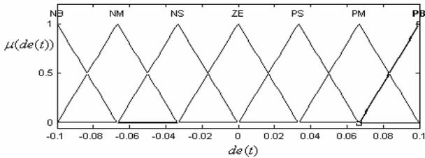
Fig. 4. Membership functions for derivation of error  $de(t)$ .
