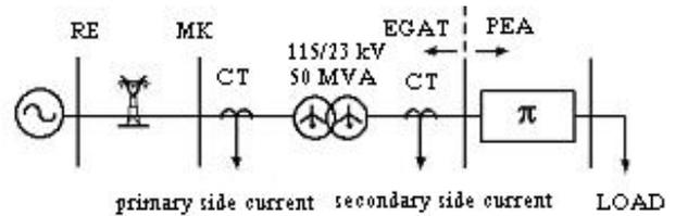
Fig. 3. The system used in simulations studies.
