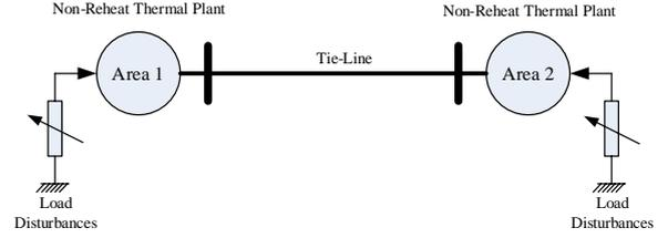
Fig. 1. Two-area interconnected power system.
