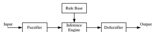
Fig. 4. Components of a fuzzy logic controller.
