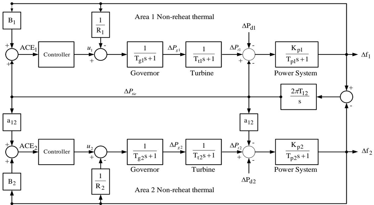
Fig. 2. Two-area interconnected power system with controller.
