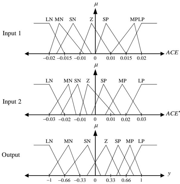
Fig. 9. Optimized membership functions for optimal FLPI controller.
