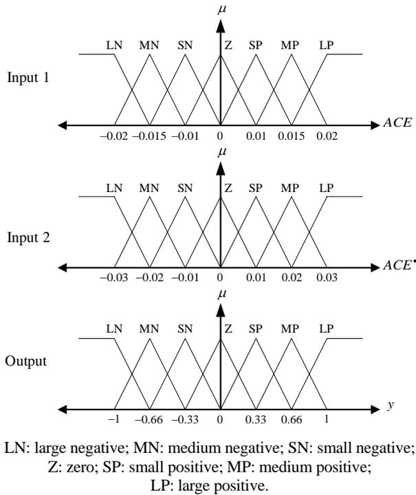
Fig. 5. Membership function for non-optimal FLPI controller.
