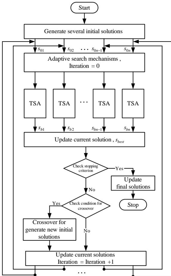
Fig. 8. Procedure of multiple tabu search algorithm.
