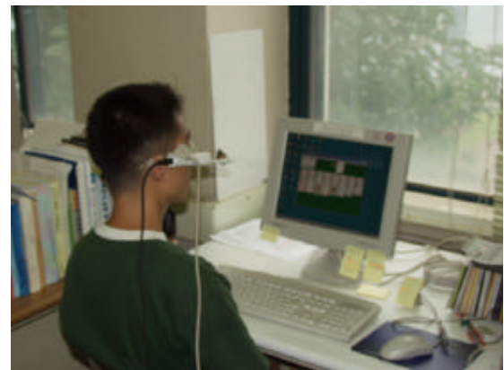
Fig. 11. A scene of playing a computer game, "freecell", by using the proposed eye-gaze tracking system.
