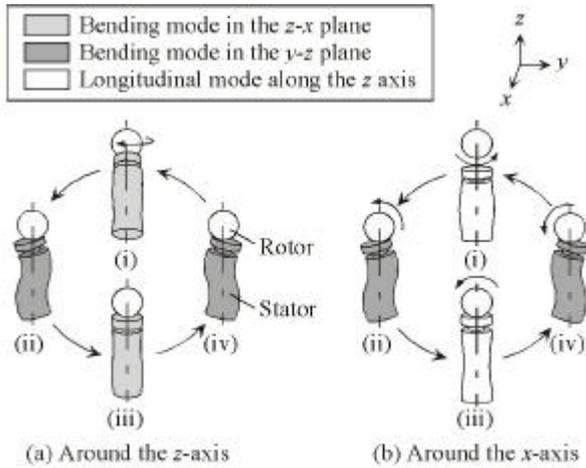
Fig. 1. Driving principle of a multi-DOF ultrasonic motor.
