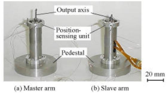
Fig. 5. Master and slave arms for active endoscope.
