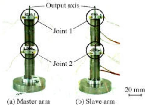
Fig. 11. Master and slave arms with two joints.
