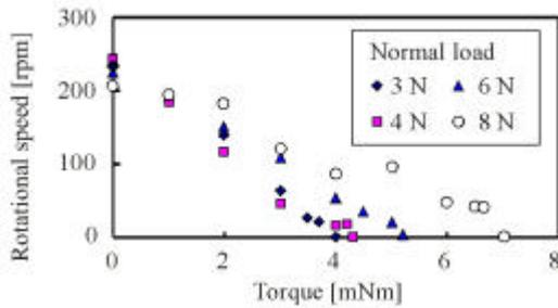
Fig. 4. Relationship between torque and rotational speed.
