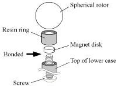
Fig. 8. Rotor/stator contract unit.
